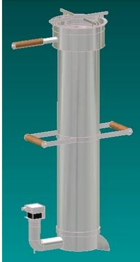
The gasifier seen here is nothing more than a vertical cylinder with a removable burner on top and a grate at the bottom. A small fan supplies air underneath the grate. On a given biomass and at a given fan speed, the diameter of the reactor determines the amount of gas produced, and the height of the reactor determines the length of time that this gas is produced.
