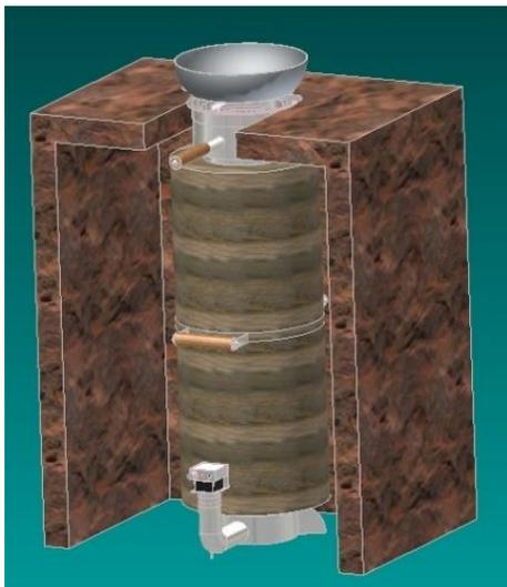
It is advisable, therefore, that the reactor not be housed, but that the gasifier be enclosed. An enclosure makes it virtually impossible for someone to accidentally knock over the gasifier. Of course it is highly recommended that the front of the enclosure be fitted with a door, not shown in the picture on the left.
